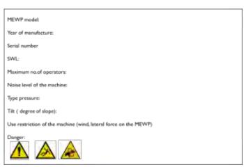
This **safety label** should be placed on the machine, in a **location that is visible to all operators**, regardless of the MEWP conditions of use (platforms raised or lowered, MEWP between rows of trees etc.). It is recommended to display this information at the front and/or rear of the MEWP, the only areas that are visible when the machine is between rows of trees.
